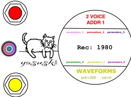
**The AutoFade mode is activated by HOLDING the top switch on the right side. The fundamental status of the AutoFade is Fixed output level. Then click the top switch on the left side start AM modulation. The modulation speed is varies from the distance between the "left hand position" and the Volume antenna.**
