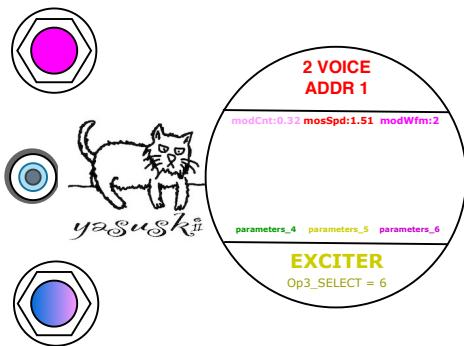
Click the upper knob to move to the LPF controller (color changes to Magenta). The lower knob changes to the effect mode selector. The fundamental is switching to the LPF cut off frequency (Indigo). The next, turn the lower knob until the LED turns to Pink to select the modulator for the LPF. Then the upper knob accepts to LFO speed.
