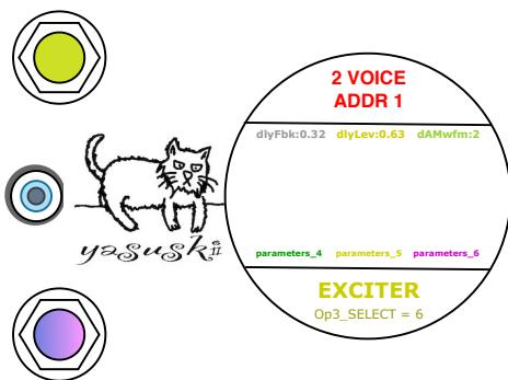
Click the upper knob to move to the Delay controller (color changes to Leaf). The lower knob changes to the parameter selector. The fundamental is switching to the Delay feedback (Indigo). Then the upper knob accept to set the values. The next, turn the lower knob until the LED turns to Leaf to select the level controller for the Delay units. Then the upper knob accepts to Delay Level .
