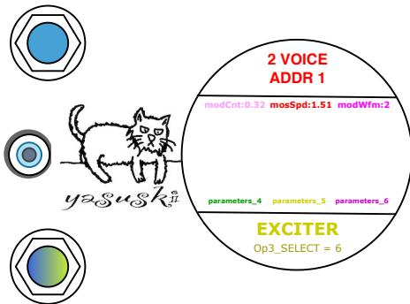
Click the upper knob to move to the LFO1/2 controller (color changes to DarkCyan). The lower knob changes to the selector for LFO1/2. The fundamental is switching to the LFO1 waveform selector (Indigo). The next, turn the lower knob until the LED turns to Leaf to select the waveform selector for the LFO2. The upper knob is reserved for the LFO waveform selectors (4 types).
