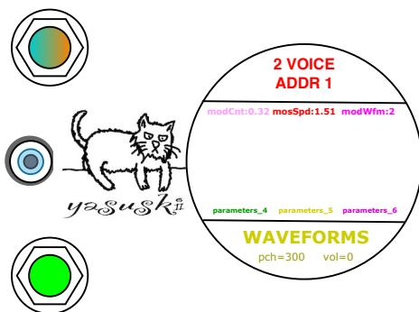
Click the lower knob once from the neutral position (yellow) to enter EXCITER mode. The LED on the upper knob lights up in SkyBlue / DarkCyan / Orange color, which means the knob is accessing to the preset selector of the EXCITER.
