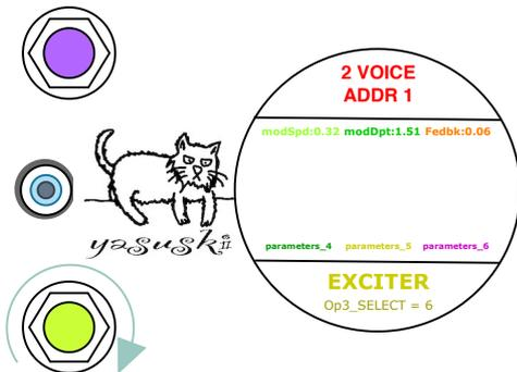
Click the upper knob to move to the LPF controller (color changes to Magenta). The lower knob changes to the effect mode selector. Turn the lower knob until the LED turns to Leaf to select the flanger. Then the upper knob accepts to LFO speed.
