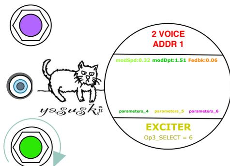
Turn the lower knob until the LED turns to Green to select the chorus. Then the upper knob accepts to LFO depth.
