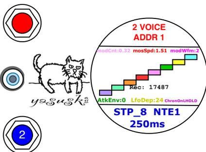
Click the lower knob then the parameter is moved to : Note pattern selector (17 preset with 15 editable notes) for the Arpeggiator. The preset notes are written in the file by the C#SV format on the microSD.
