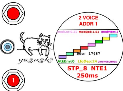
Click the lower knob then the parameter is moved to : Pattern selector (Up / Alternate / Down / Random) for the Arpeggiator.
