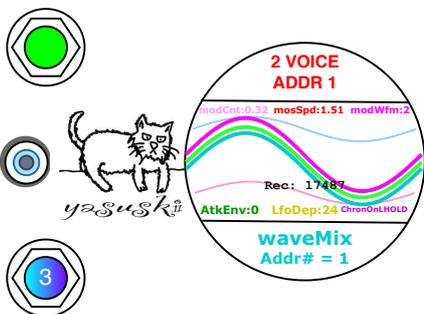
Click the lower knob then the parameter is moved to : Waveform Mix Selector / Edit mode. (the 14 preset with 18 editable waveform mix) The parameters (32 wavetables with 5 levels) controlled by the upper knob is changed by clicking the upper knob, then turning the knob for selecting / changing the values.
