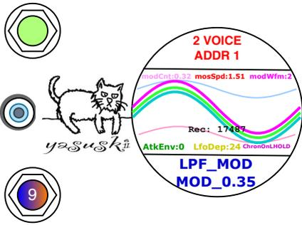
Click the lower knob then the parameter is moved to : LPF Frequency / LPF Modulation / Flanger / Chorus / Dub Rate controller mode.
