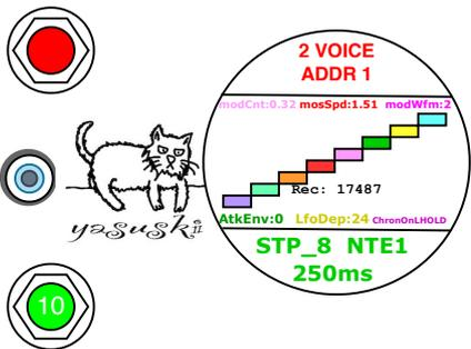
Click the lower knob then the parameter is moved to : speed control for the Arpeggiator.
