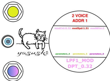
The fundamental position of the upper knob is switching to the LPF cut off frequency (Indigo). The lower knob accept the parameter of the cut off frequency for the LPF. The next, turn the upper knob until the LED turns to Pink to select the modulator for the LPF. Then the lower knob accepts to LFO1 speed.
