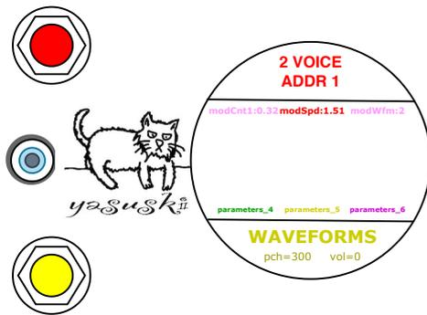
For easy accessing, the LPF has the another controllers. Click 5 times the lower knob from the neutral position (Yellow) to enter LPF\_MOD mode. The LED on the upper knob lights up in Leaf, which means the knob is accessing to the parameters for the FILTERS.
