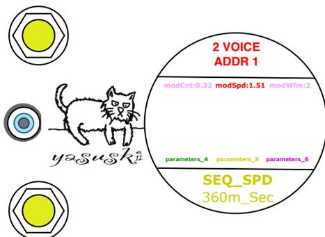
If the SEQUENCER mode is selected, this page is assigned to SEQ\_SPD. Move to EXCITER page for access to the filter controllers.
