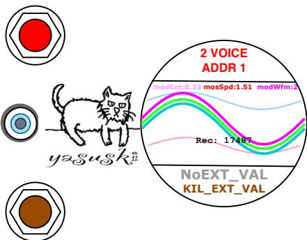
Turn the lower knob clockwise then the LED on the lower knob lights up in Brown, which means the knob is activating the mode "NoEXT\_VAL with KIL\_EXT\_VAL".
