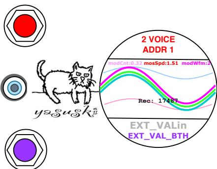
Turn the lower knob clockwise then the LED on the lower knob lights up in Violet, which means the knob is activating the mode "EXT\_VALin with EXT\_VAL\_BTH".
