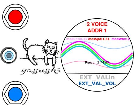
Turn the lower knob clockwise then the LED on the lower knob lights up in Indigo, which means the knob is activating the mode "EXT\_VALin with EXT\_VAL\_VOL".
