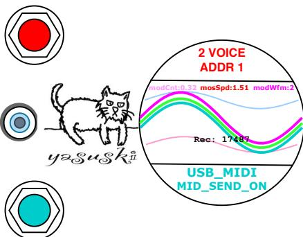
**Turn the lower knob clockwise then the LED on the lower knob lights up in DarkCyan, which means the knob is activating the mode "USB\_MIDI\_OUT with NO\_BIAS\_SHIFT".**
