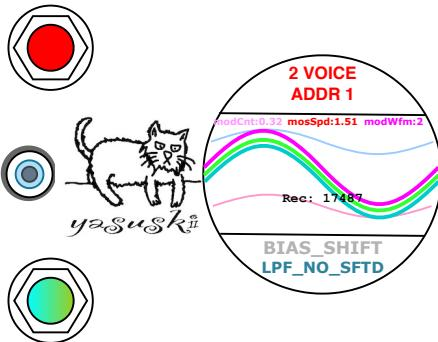
**Click the lower knob 4 times from the neutral position (yellow) to enter BIAS\_SHIFT mode. The LED on the lower knob lights up in Cyan, which means the knob is accessing to the mode selector of the LPF / HPF/ BIAS\_SHIFT / USB\_MIDI / Input Selectors.**
