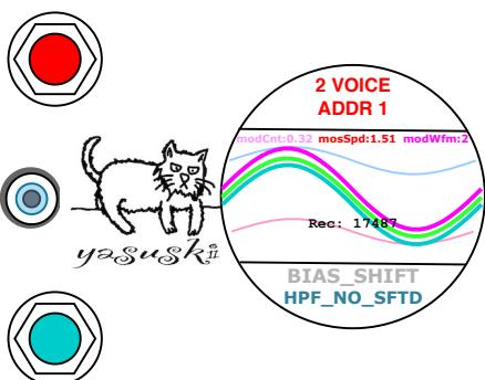
**Turn the lower knob clockwise from the neutral position "LPF with NO\_BIAS\_SHIFT". The LED on the lower knob still lights up in Cyan, which means the knob is activating the mode "HPF with NO\_BIAS\_SHIFT".**
