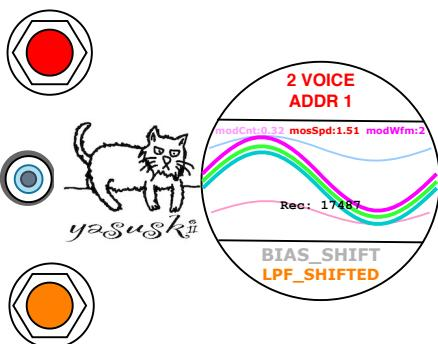
**Turn the lower knob clockwise then the LED on the lower knob lights up in Orange, which means the knob is activating the mode "Distorted signals with BIAS\_SHIFT". The BIAS\_SHIFT is analog circuit not coding on the software, which is activated by the analog switches.**
