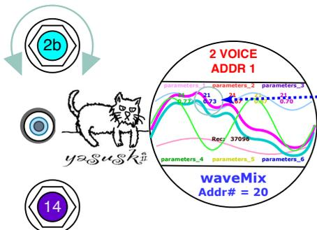
Access to the parameter "OSC2 waveform selector" by clicking the upper knob (forward) once. The LED turns to SkyBlue.
