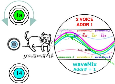
The Mix Out is a selector for the memory set which contains the combinations of the parameters, waveform selector and output level controller for the Oscillators. The Mix Out has 32 address. **The first 14 is the "Preset" group (LED = SkyBlue).** Access to the Mix Out Selector on the lower knob by double clicking (backward) from the neutral position (Yellow).
