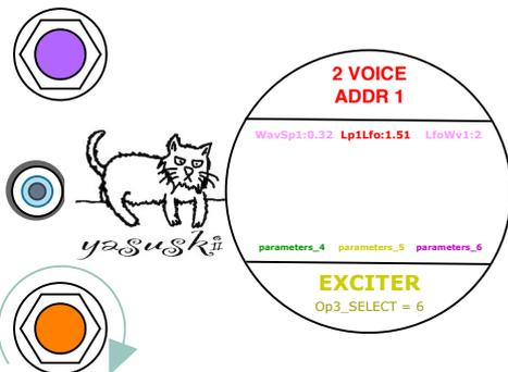
Turn the lower knob until the LED turns to Orange to select the chorus. Then the upper knob accepts to LFO speed.
