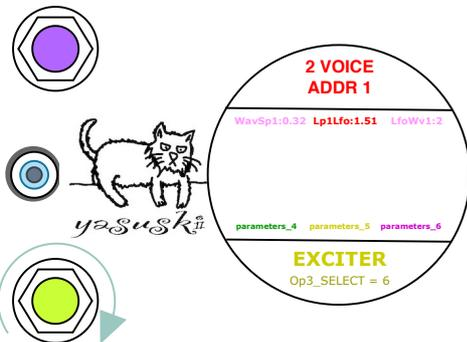
Click the upper knob to move to the LPF controller (color changes to Magenta). The lower knob changes to the effect mode selector. Turn the lower knob until the LED turns to Leaf to select the flanger. Then the upper knob accepts to LFO speed.
