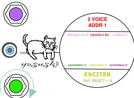
Turn the lower knob until the LED turns to Green to select the chorus. Then the upper knob accepts to LFO speed.
