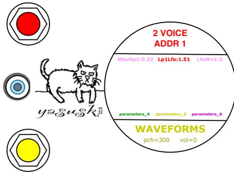
Click the lower knob from the neutral position (yellow) to enter EXCITER mode. The LED on the upper knob lights up in SkyBlue / DarkCyan / Orange color, which means the knob is accessing to the preset selector of the EXCITER.
