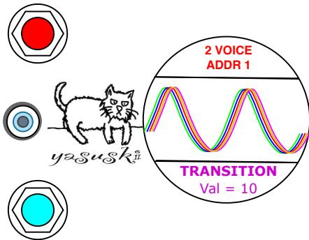
**Turn the lower knob for switching the Transition Waveform. Then the LED color on the lower knob lights up in Cyan .**
