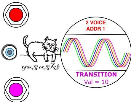
**Click the lower knob then the parameter is moved to : the Transition Waveform switcher.**
