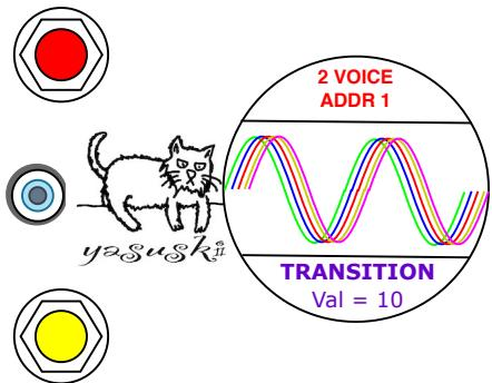
**Click the lower knob twice from the neutral position (yellow) to enter TRANSITION mode. The LED on the upper knob lights up in Magenta color, which means the knob is accessing to the parameter of the TRANSITION.**
