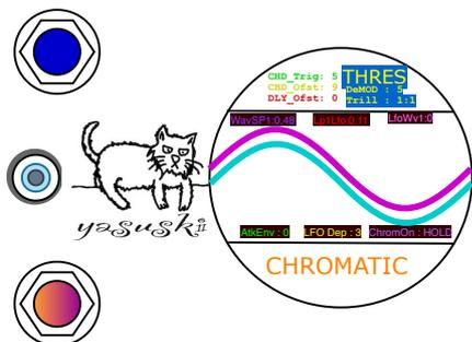
Turn the lower knob clockwise to enter CHROMATIC mode. At this time, the upper knob is assigned to a parameter that sets the delay time magnifier, DLY\_Ofst = pot00g.
