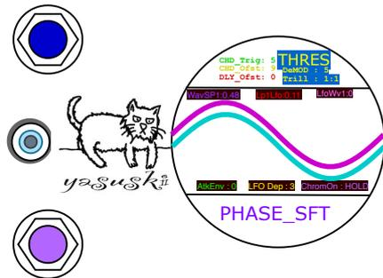
Turning the lower knob clockwise will enter pitch bend/phase shift mode.
