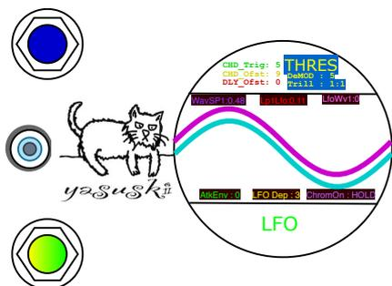
Turn the lower knob clockwise to enter LFO mode. At this time, the upper knob is assigned to a parameter that sets the starting address for the Chord Sequencer, CHD\_Ofst = pot0.
