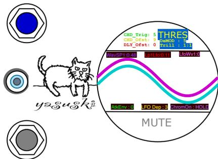
Turn the lower knob clockwise to enter MUTE mode. At this time, the upper knob is assigned to the trill note pattern selector pitch\_drift = pot00v.
