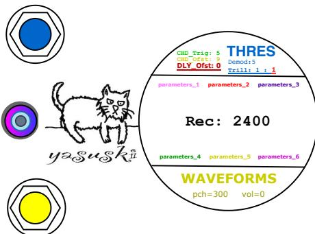
**The looper capture time follows the tempo and steps of the Arpeggiator.** For example,  $25\text{ms} * 4\text{steps} * 24(\text{magnification}) = 2400\text{ms}$ . The magnification is set by **DLY\_Offset** in **TRES / CHROMATIC** mode. The recording duration is shown at the center of the LCD, then start count down after the Looper start recording.
