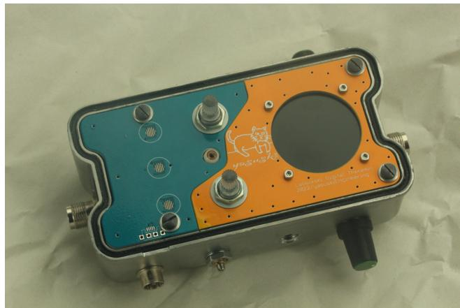
LaVoixski is a digital musical instrument based on the Theremin. It has the RF oscillation circuits "The heart of the Theremin", but does not have the analog demodulators for produce the audio signals.
