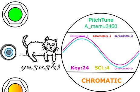
The Chromatic mode is available on all voicing modes. Access to the parameter "MUTE Switch" on the lower knob as the power-on neutral position (Yellow). Rotate the lower knob clockwise 3 notches then the LED color on the upper knob turns **Leaf** and lower knob turns **Orange**.
