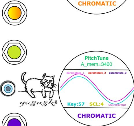
When the **PitchTune** mode is selected with the upper knob, the upper knob is assigned to the parameter that sets the activation time of the chromatic mode. Then the LED color on the upper knob turns to **Leaf**. When the Chromatic mode is inactivated, the LED on the lower knob turns **Purple**.
