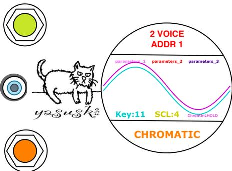
Click the upper knob twice, then moving to the **2 voice mode**. The upper knob has been working for the scale selector at this time. The color of the upper knob is still colored in **Leaf**. The 32 preset scales are available.
